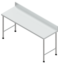
PRODUCT IMAGE · Rendered E25144(112-1800x0600): 1800 x 600 mm, 900 mm working height, 150 mm rear splashback, 1050 mm overall height; no undershelf.
