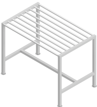
PRODUCT IMAGE · Heavy duty Grade 304 stainless steel pot drying rack with tubular drying surface, cross-braced frame and stainless steel adjustable feet. 1200mm x 750mm model shown.
